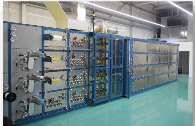
The masterpiece from Benninger offers excellent convertibility from laboratory to production scale. In addition, the Laboratory machine offers the possibility to conveniently test new processes, recipes and processes.
